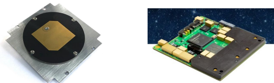
Fig. 24: Space segment communication hardware: (left) ISISPACE S-band patch antenna; (right) NANOLink SDR S-band transceiver. [25][26]
